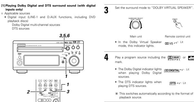
Main unit Remote control unit • In the Dolby Virtual Speaker DD VS - Lit mode, this indicator lights. Play a program source including the or dits • The Dolby Digital indicator lights IDD DIGITAL - Lit when playing Dolby Digital • The DTS indicator lights when |DTS - Lit playing DTS sources. \* This switches automatically according to the format of the
